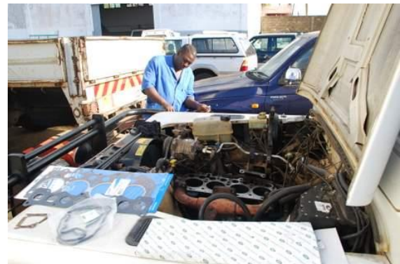
Repairing the head gasket
